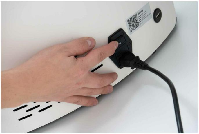
Before turning on the printer, make sure that the power supply cable is connected properly. It is a standard three-wire cable with a standard connector used in computer power supply units.
