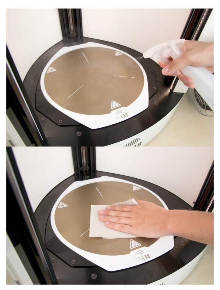
Tip: Make sure the PrintPad is always degreased properly and thoroughly before every printing session. The PEI printing surface is versatile and very durable but it is very sensitive to grease. If the surface is not degreased properly, problems with lower material adhesion may occur.
