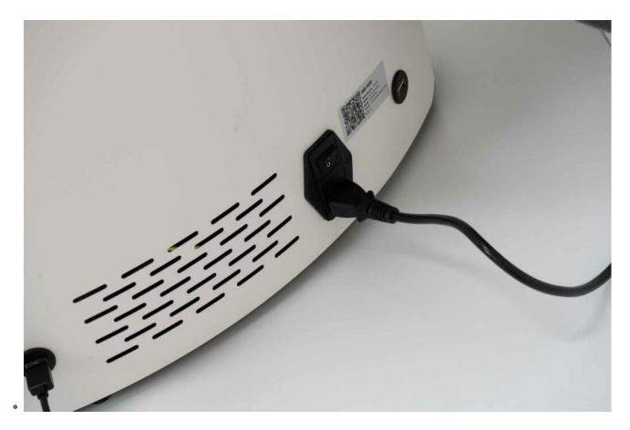
Turn on the printer by switching the rocker switch on. The machine's successful start and readiness
