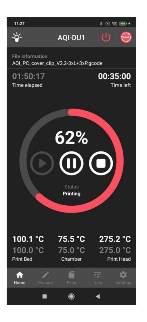
At the top there is a common line for all tabs. On the left there is an icon for turning on/off the lights, in the middle is the name of your printer and in the right-hand corner you can see the *EMERGENCY STOP* button, which you can use to stop the machine while printing is in progress. The printer is then restarted and after a short time it is prepared for other tasks. By pressing this button, the printing in progress is stopped and it is not possible to continue it later.
