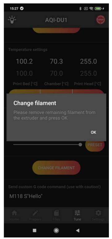
Insert the new filament in the extruder so that there is about 1cm of the filament in the Bowden and press *LOAD*.
