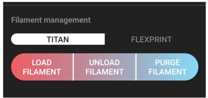
Note: If you are loading filament whose melting temperature is higher than 250 °C, set the required temperature manually (see the instructions 2 paragraphs below) and then select the macro command.
