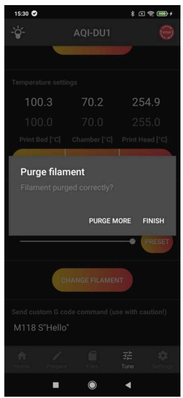
At the end it is necessary to remove all the extruded filament from under the nozzle; once you press *OK*, the printing will continue.
