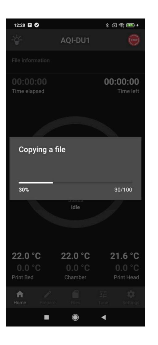
You can remove the USB disk during the printing without affecting the printing process in any way. Once the printing is completed, the file is stored in Internal->USB file.
