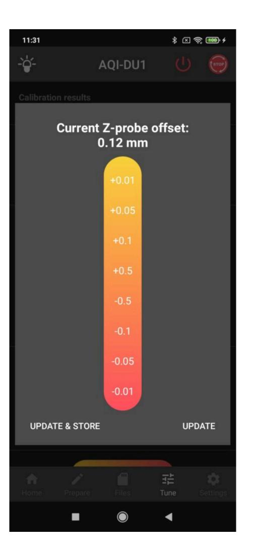
Note: When decreasing the offset value, you have absolute control over the printer, so you must proceed very carefully. We recommend using values -0.05 and -0.01 mm.
