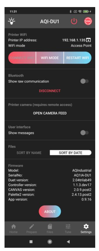
As standard, the printer looks for known Wi-Fi networks in the vicinity and tries to connect to them. The *Auto* and *Client* modes are used for this. While in the *Auto* mode the printer tries to connect to the network and switches to the *AP* mode if a connection cannot be established, in the *Client* mode it keeps trying to connect to the network.
