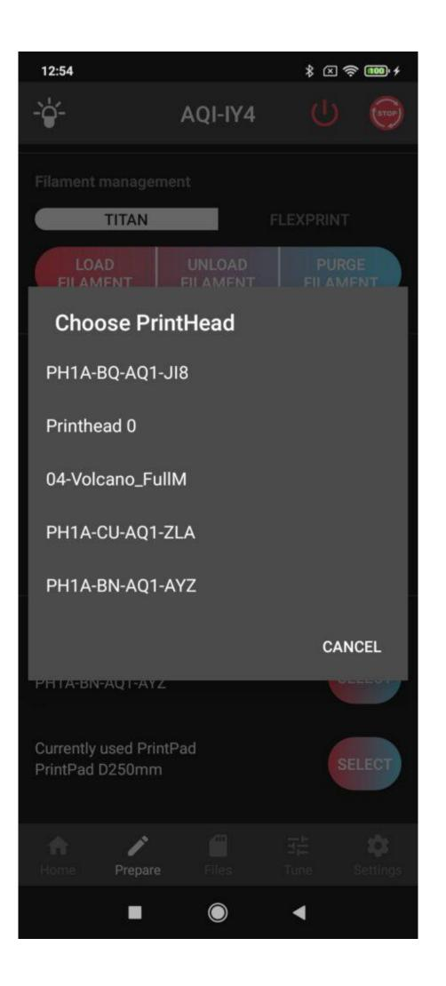
After the first such change, offset is set to 0.0mm. Therefore it is necessary to fine-tune the **Height of** the first layer during the first use of the new accessories.
