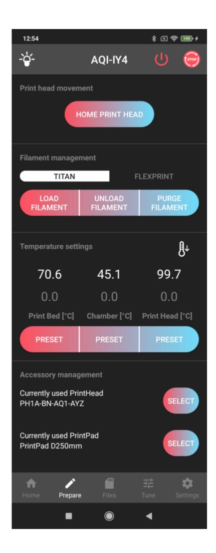
The *HOME PRINT HEAD* button is used for putting the print head in the initial position (e.g. after printing is stopped).
