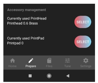
If you want to use the accessories, replace it according to the instructions (How to replace the print head) and use the *SELECT* button to choose the accessories from the list. After each such change, the pre-set figures (e.g. offset) of the accessories are loaded and automatic calibration is done before the
