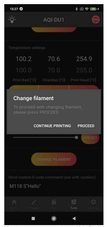
After that you must remove the rest of the filament manually and continue by pressing OK.
