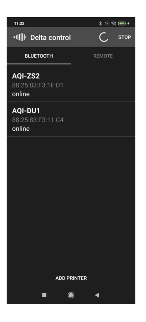
You can add more printers on this initial screen. After pressing *ADD PRINTER* button, the camera is turned on to scan the QR code. The code is located in the back part of the printer, near the power supply cable.
