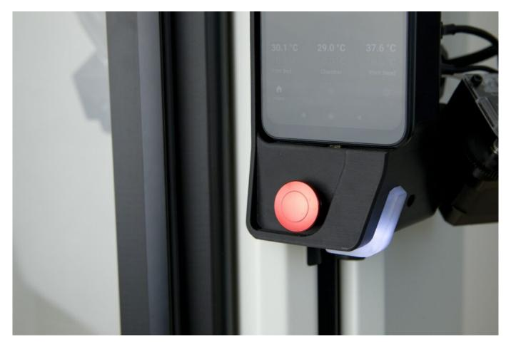
The printer is restarted completely and is then ready for operation again. However, before that it is necessary to remove from the pad any material whose printing has been interrupted and prepare the pad again. If the printer shows unusual performance or damage or if any of its parts have disintegrated, please contact the supplier's service department.
