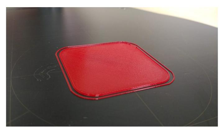
A layer that is too low has scratches in it cause by the nozzle movement and these scratches can be felt to the touch. If this situation occurs, in the DeltaControl application on the **Tune tab**, increase the Z-offset value using, for example, the +0.05 mm button.
