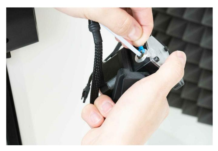
Then insert the extruder into the corresponding recess in the hub. Place the extruder in the hub with a light push.
