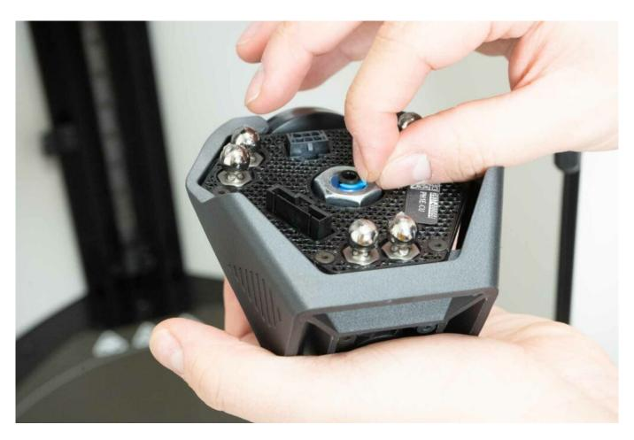
Insert the bowden fully into the printhead.
