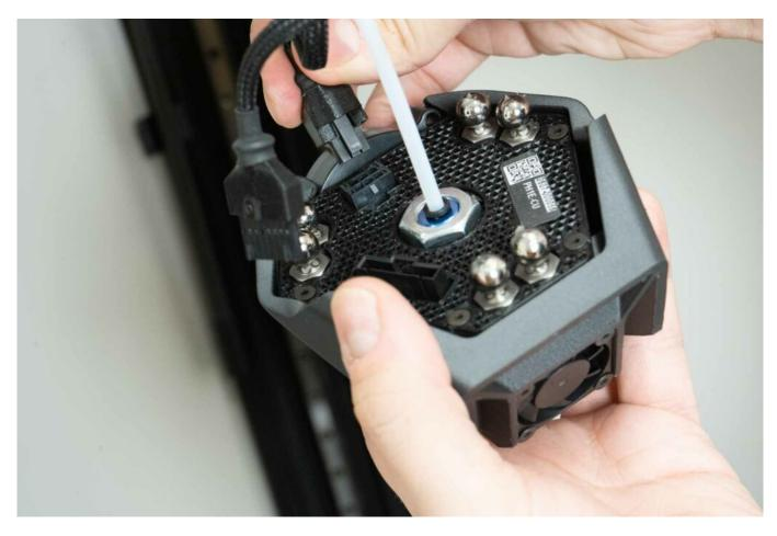
Put back the blue clip to secure the bowden.
