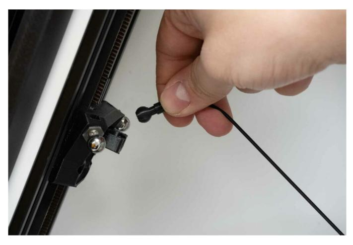
Carefully release the arms from the transport holder printed from flexible material.
