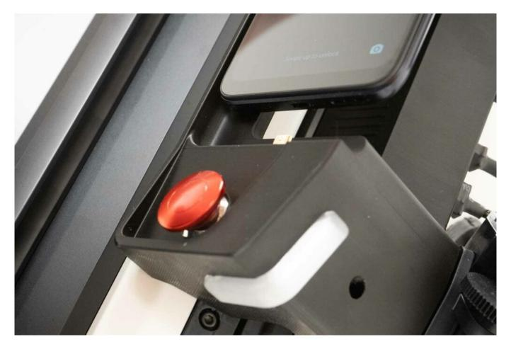
Warning: The only correct direction of positioning the display is vertically from above. Approaching in a different direction other than this may damage the charging cradle connector. Please use the same caution when removing the display.
