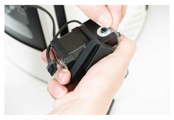
Now insert the bowden fully into the extruder.
