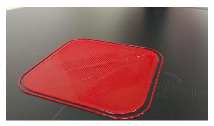
The opposite extreme, too high first layer, is typical by gaps between the lines, perimeters and poor adhesion. If this is happening, in the DeltaControl application in the **Tune tab**, reduce the Z-offset value, using, for example, the -0.0.5 mm button.
