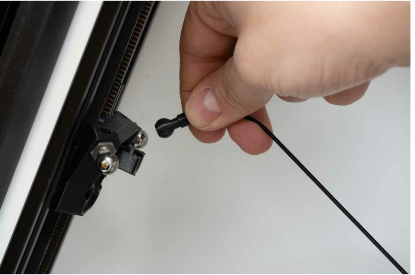
Carefully release the arms from the transport holder printed from flexible material.
