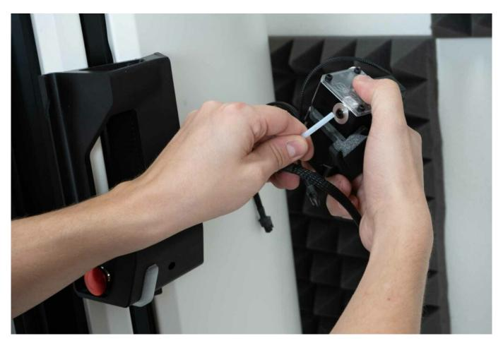
Put the blue clip back onto the extruder.
