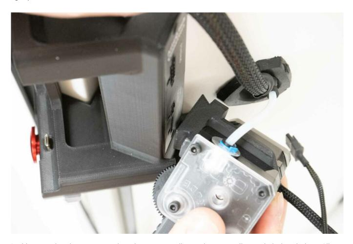
In this step, plug the connectors into the corresponding sockets according to their descriptions. All connectors are unique so they can be connected in only one way.
