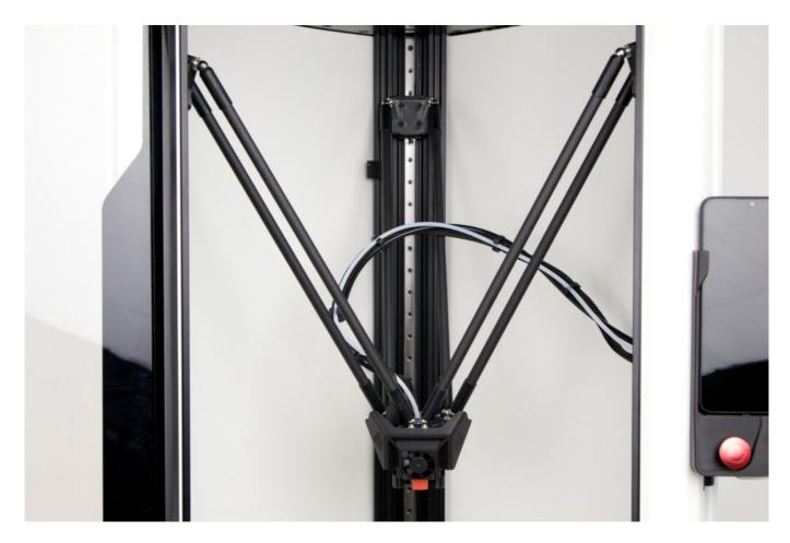
Warning: Before releasing the printhead, check that all magnetic connections are secure by pulling gently.
