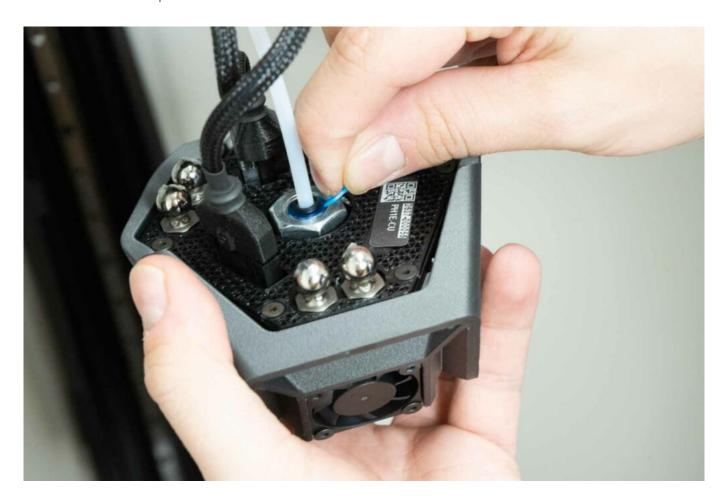
Position the printhead so that the FRONT is facing you and gradually begin to fit the arms onto the magnetic joints while holding the printhead with your other hand.
