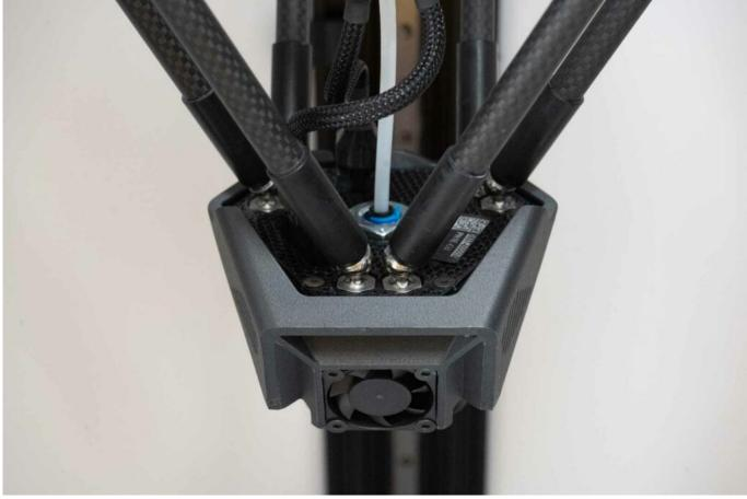
Warning: The cable harness must be routed between the rear and right pair of arms, as shown in the figure below.
