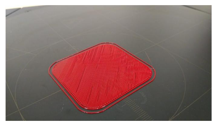
Warning: During the decreasing the Z-offset, be very careful not to reduce it too much, the nozzle could hit and scratch the printpad.
