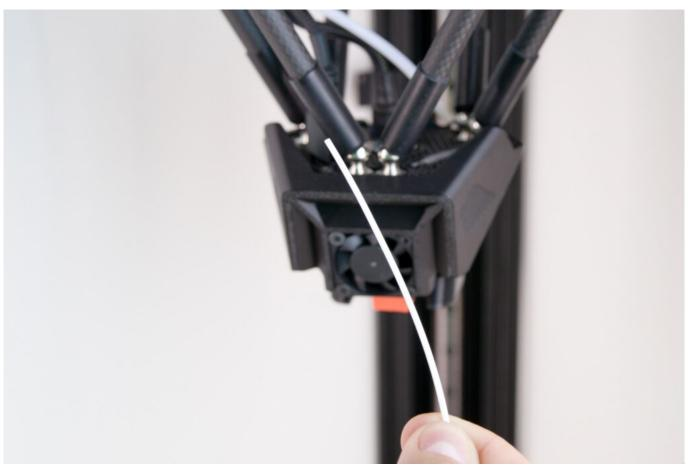
Once the nozzle has reached the desired temperature, insert the cut piece of filament into the print head. Melted filament should start flowing out of the nozzle.
