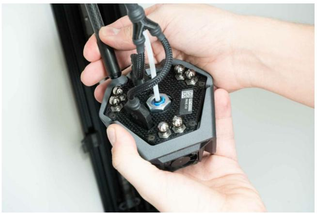
Then carefully disconnect the Bowden (take out the blue clip and push the black collet towards the printhead) and both connectors.
