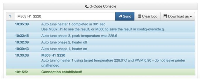
Note: During temperature calibration, the nozzle is heated to more than 220 °C, so be very careful with regard to your personal safety. Also, do not perform any other operations, otherwise, the calibration will not be performed properly.
