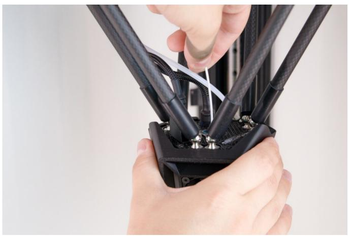
Note: At this moment, do not leave the filament in the nozzle for longer than necessary and continue immediately.
