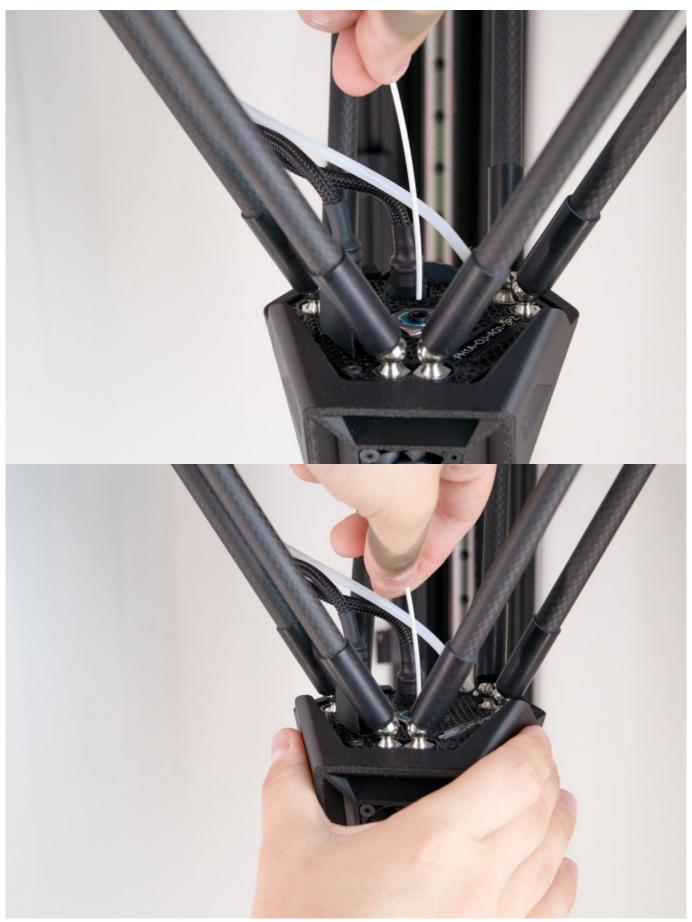
Tip: If no filament flows out of the nozzle, the nozzle is likely to be clogged and the cold pull method will probably not work. In such a case we recommend replacing the nozzle with a new one.
