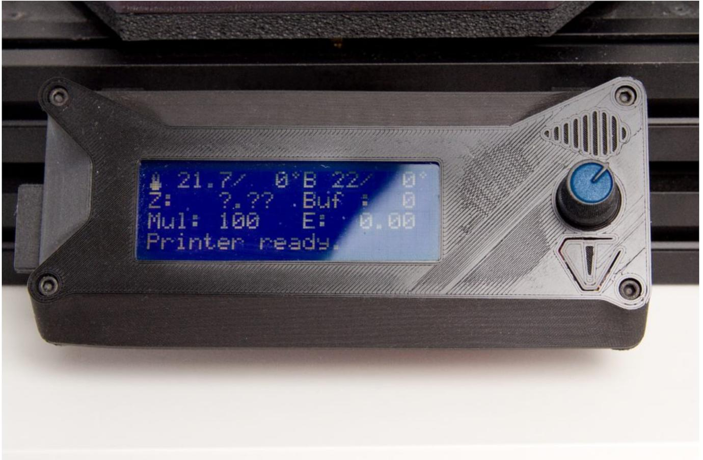
You can spin the wheel up and down and thereby move around in the menu, set the printer's temperature, or even manually control the motion of its motors. You can also press it to confirm menu choices or enter submenus.
