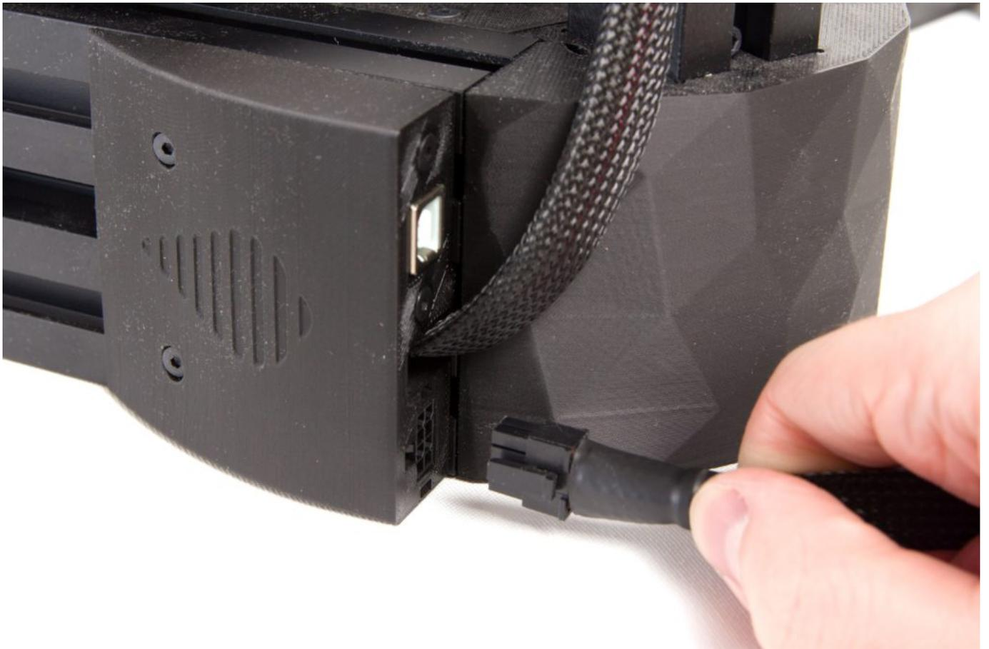
Caution: It is important that the cable from the printer not be bent, folded, or otherwise deformed.
