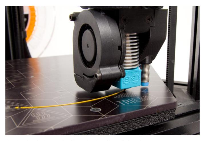
Then the printer begins extruding filament based on the supplied G-code.
