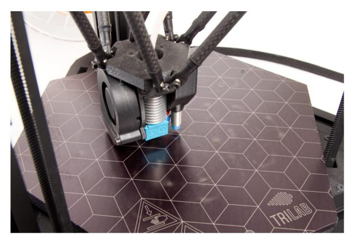
After calibration is completed, the head will park in the front part just above the base and begin heating the nozzle along with the inserted filament.
