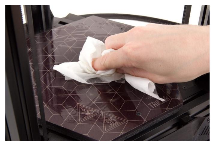
Use the same grease-removal procedure if you plan to print using ABS or a similar material.
