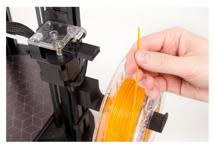
2) Remove the filament from the side of the spool and cut the filament at about 45° using the supplied pliers.
