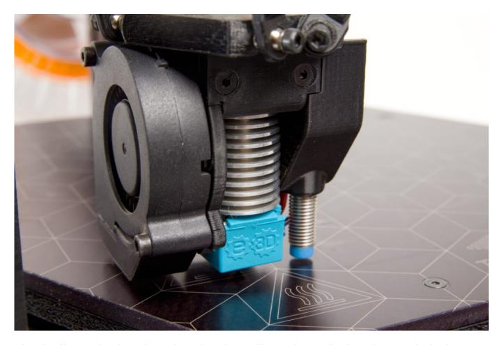
After the filament has been heated up, the printer will extrude a smile-shaped pattern in the front part of the bed. The purpose of this print is to stabilize the pressure in the nozzle and wipe away any grime that is nearby the nozzle.
