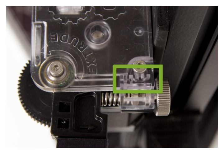
If there are significant leftovers from the filament on the feeder wheel, this may mean excessive pressure. To fix this problem, loosen the screw slightly (via clockwise rotation).
