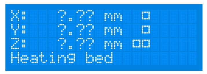
The second screen shows information on current X, Y and Z coordinates of the printhead.
