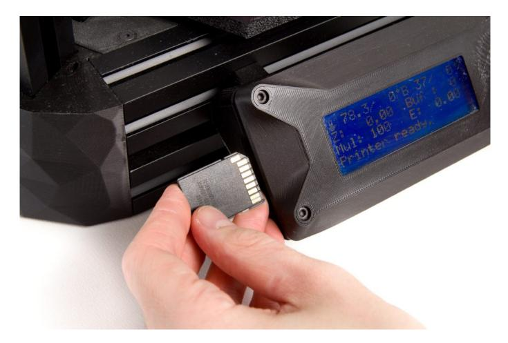
After the card has been inserted into the printer (or pulled out and re-inserted), the card's contents are listed on the display. Use the control wheel to place the cursor over the file of your choice, and then press the control wheel to begin printing.
