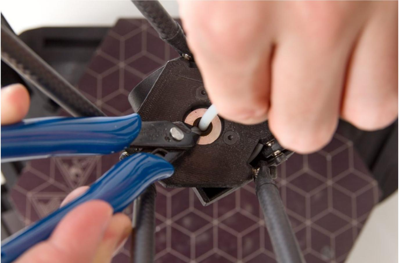
Remove the Bowden cable from the print head.
