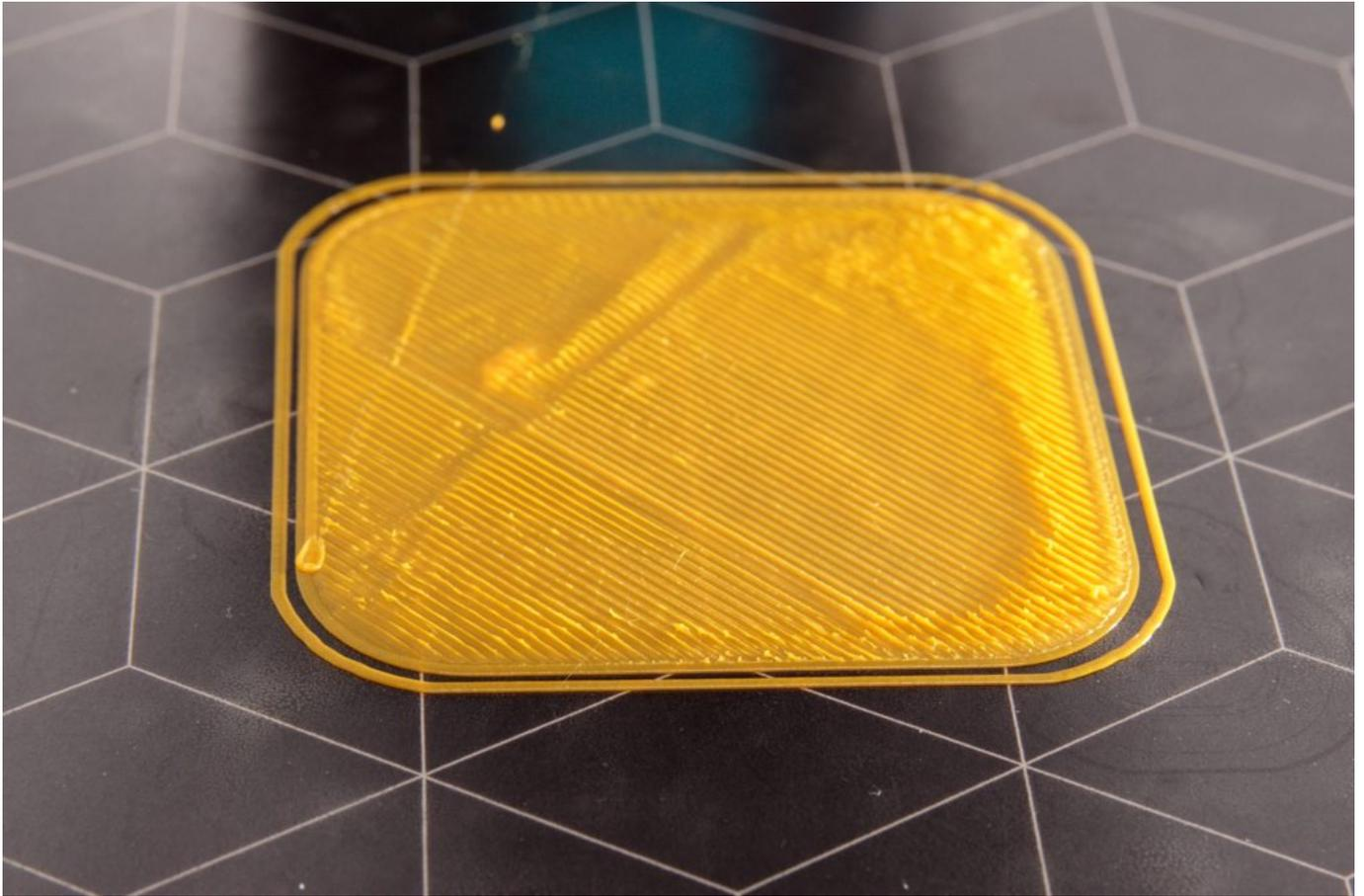
The second possibility is that the first layer is too low. Here the solution is to raise the first layer. Proceed according to The First Layer Has Insufficient Adhesion above. However, here you will be adding to the Z-babystep value and then lowering the Z-probe-hgt value by the same value that you added in Z-babystep.
