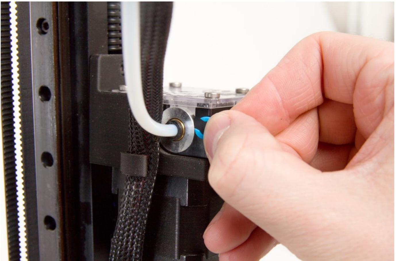
You can use your fingers or pliers to apply pressure on the black collet ring. However, make sure not to damage the bowden tube with the pliers.
