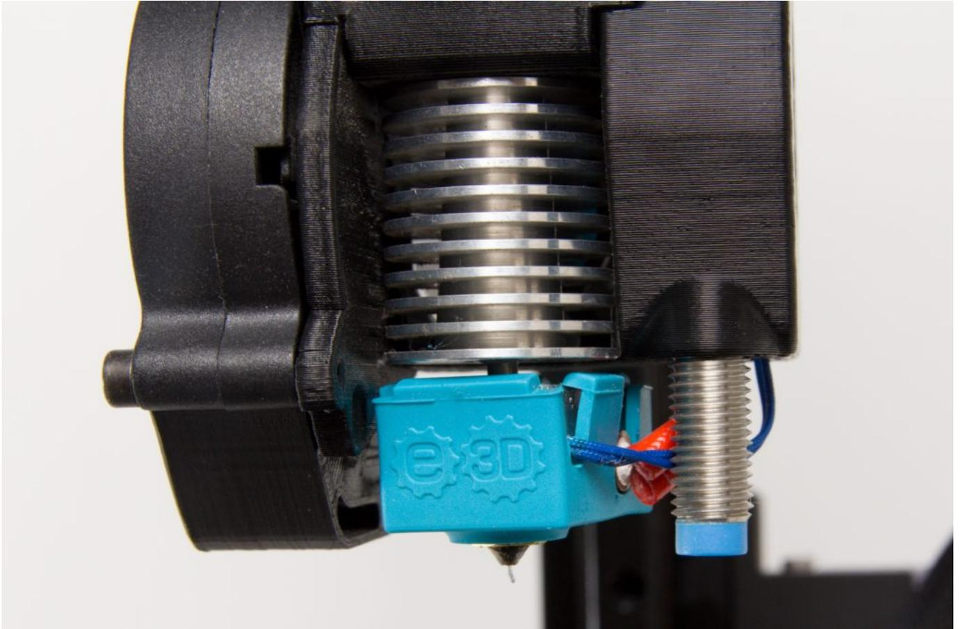
Follow the steps from Filament Is Leaking Over the Heat Block above. After removing the hot end, straighten the block's rotation and place the hot end back into the print head using the same instructions.
