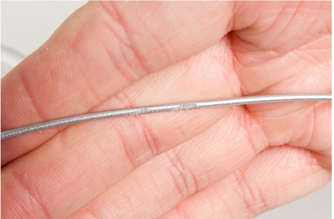
If the filament is not being moved towards the print head during the extruder's motion, the problem probably lies in an incorrect tensioner adjustment or a clogged nozzle. This problem can be accompanied with a clattering sound, and planed-off filament will appear nearby the feeder wheel. Clean and/or exchange the nozzle. Perform the "cold pull" nozzle cleaning procedure or exchange the nozzle.
