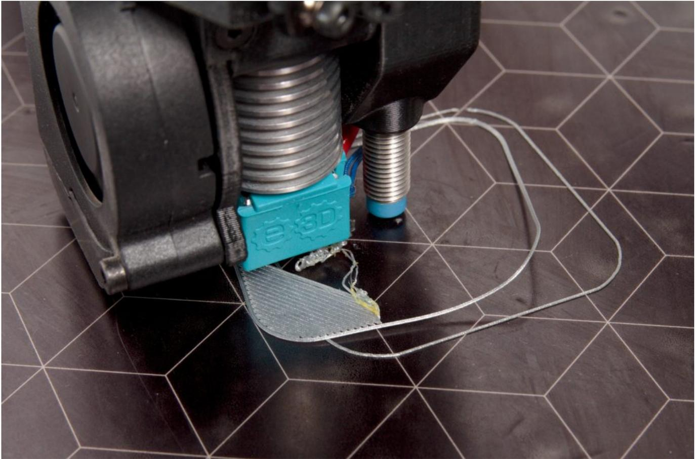
Outside of improper printing temperatures, the most common problem here lies in poor removal of grease from the base. In this situation, prepare the base thoroughly, following the Pre-print Base Preparation instructions.
