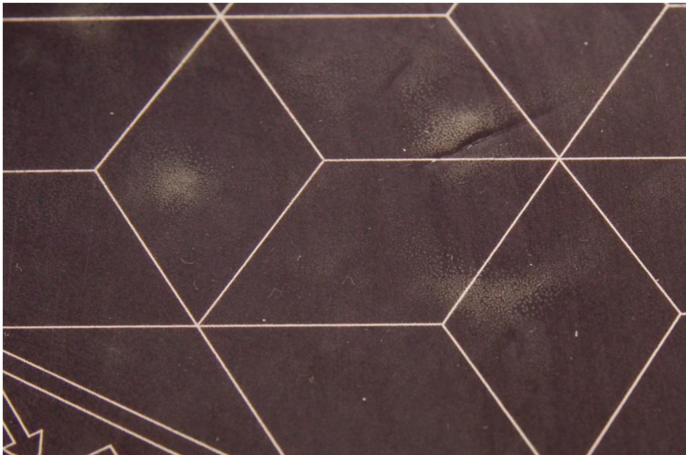
These are naturally occurring glue bubbles that appear after heating and especially after repeated printing on the same place. When the printer is being used correctly in accord with the manual, there is no need to worry about them; they will disappear on their own after some time.
