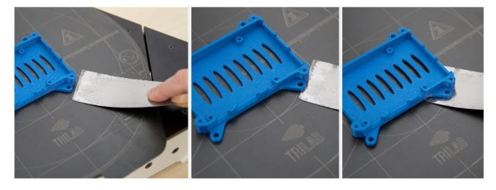
Tip: If your printed object has corners or sharp edges, this is the optimal place to slide the spatula under. Conversely, the round parts of the models are less suitable.
