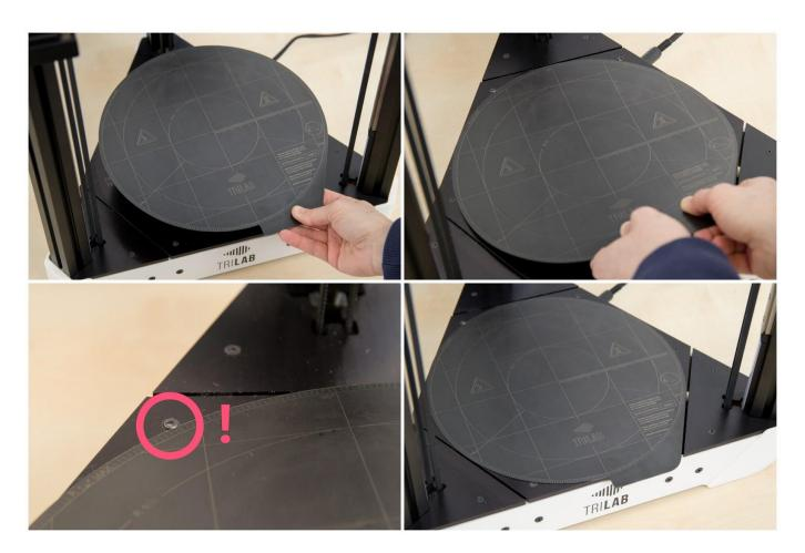
Tip: Don't worry about the PrintPad being slightly rotated. This has no effect on function.
