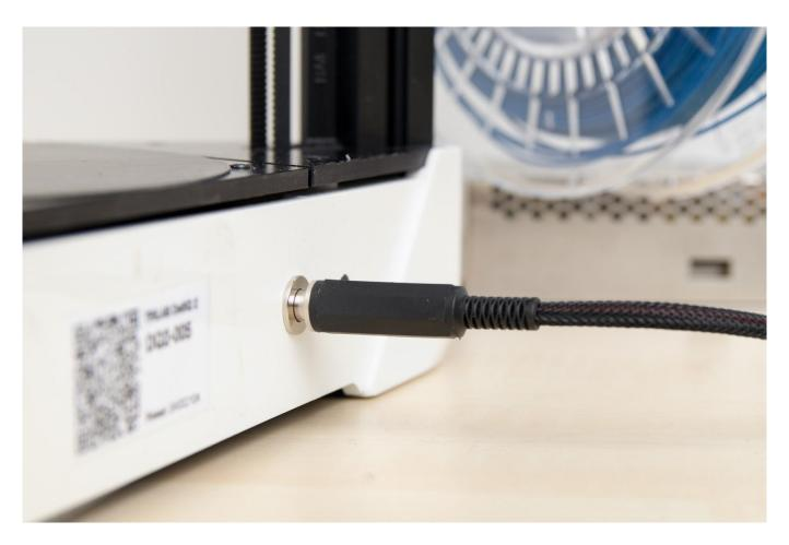
Caution: Do not bend or twist the power cord from the power supply to the printer unnecessarily nor tie it with quick-release straps.
