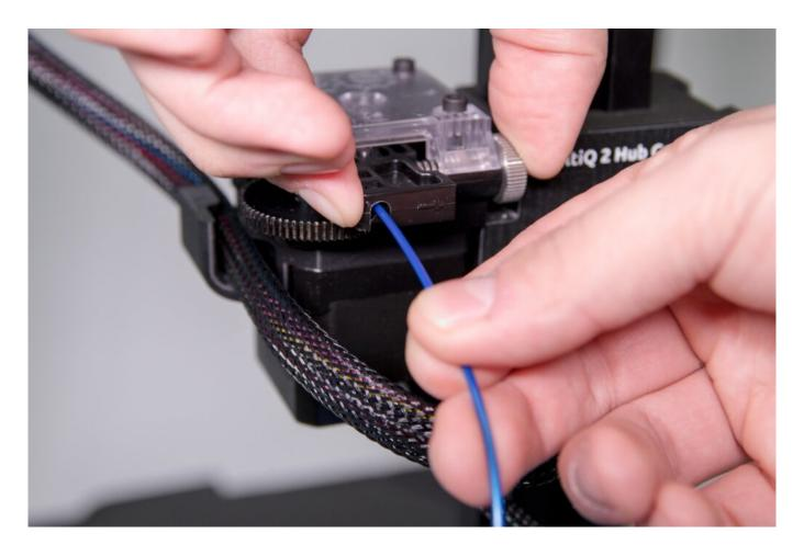
4. If your package includes a filament sensor, feed the end of the filament through the filament sensor to the extruder. If this sensor was not included, feed the end of the filament directly into the extruder.
