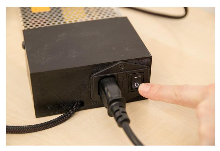
Caution: If you turn the printer off (rocker switch on the power supply) and will not be using it for an extended period of time, you should also turn off the DeltaControl display. This will prevent any problems with the phone battery.
