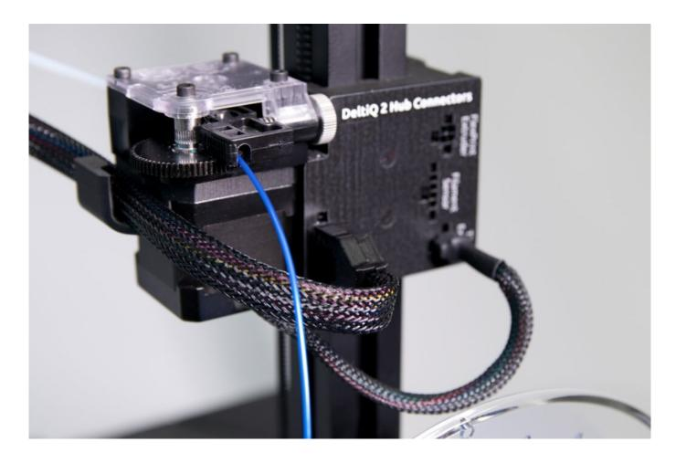
5. The end of the filament will appear in a transparent bowden duct after the extruder. When you see about a centimeter of filament in the tube, release the second-hand grip, the filament is ready to be loaded using the printer control.
