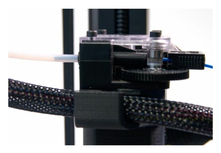
6. Have the DeltaControl display ready in-hand and select the Prepare tab, make sure the Titan is highlited and press the *LOAD FILAMENT* option.
